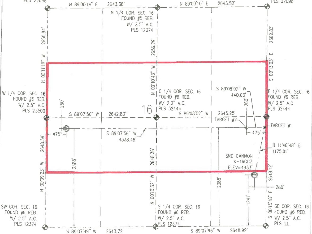
**N** IN ACCORDANCE WITH A REQUEST FROM CRAIG RASMUSON - SYNERGY RESOURCES, BASELINE ENGINEERING CORP HAS DETERMINED THE LOCATION OF THE SRC CANNON K-16CHZ TO BE 1241' FSL AND 280' FEL, AS MEASURED AT NINE-TY (90) DEGREES FROM THE SECTION LINE OF SECTION 16, TOWNSHIP 4 NORTH, RANGE 6E WEST AND THE BOTTOM HOLE LOCATION TO BE 2388' FSL AND 475' FWL OF SECTION 16, TOWNSHIP 4 NORTH, RANGE 6E WEST, 6TH PRINCIPAL MERIDIAN, WELD COUNTY, COLORADO
