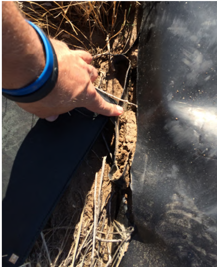
Photograph 9: 6-inch long rip observed along anchor trench in northwest corner.
