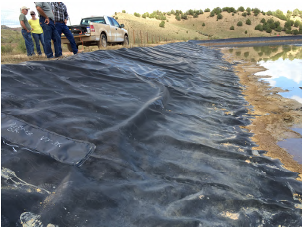
Photograph 5: View of location where a geomembrane samples were removed for testing by TRI Laboratories. Note the locations are above high water mark denoted by the lighter stained liner to the right.
