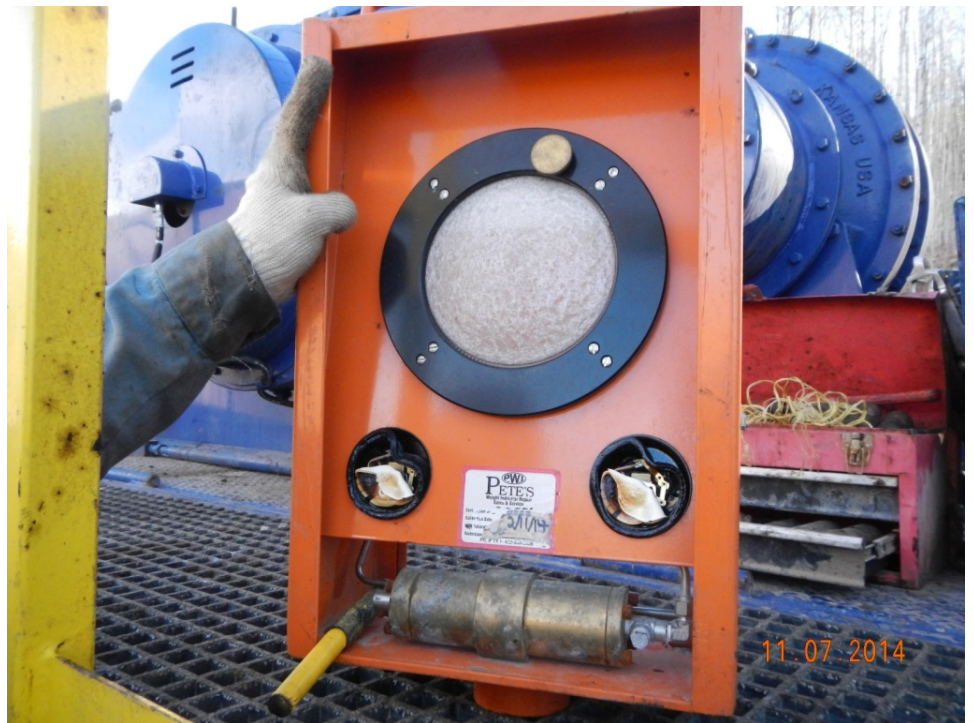
Damaged load indicator.
