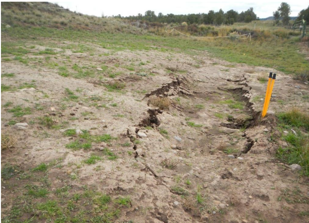
Photo 1. View of subsidence along what appears to be a pipeline tie, from the southern edge of the project area facing southward.
