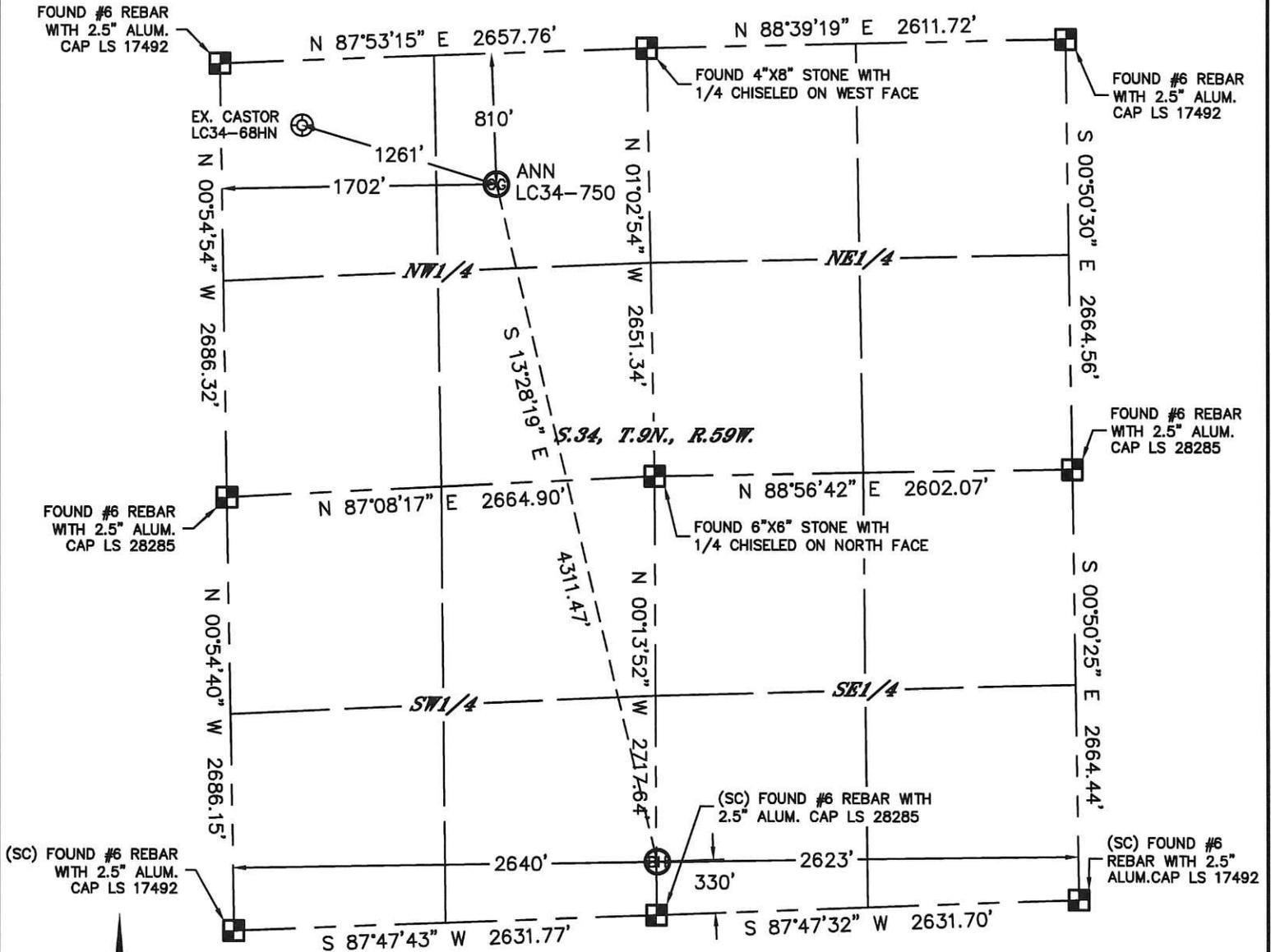
In accordance with a request from Brian James with Noble Energy Inc. Lat40°, Inc. has determined the surface location of the ANN LC34-750 to be 810' from the NORTH line and 1702' from the WEST line and the bottom hole to be 330' from the SOUTH line and 2623' from the EAST line as measured at right angles from the section lines of Section 34, Township 9 North, Range 59 West of the Sixth Principal Meridian, County of Weld, State of Colorado.
