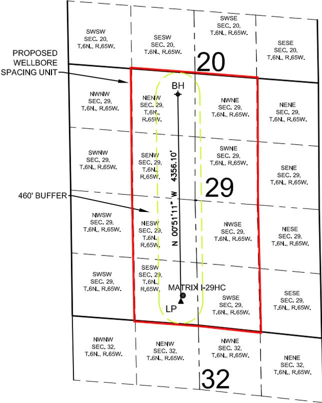
WELL **MATRIX I-29HC** TO BE LOCATED 598' FSL AND 2328' FWL, SEC. 29, T6N, R65W
