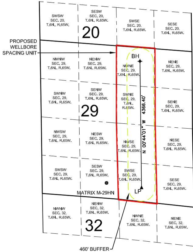
WELL **MATRIX M-29HN** TO BE LOCATED 528' FSL AND 2224' FWL, SEC. 29, T6N, R65W
