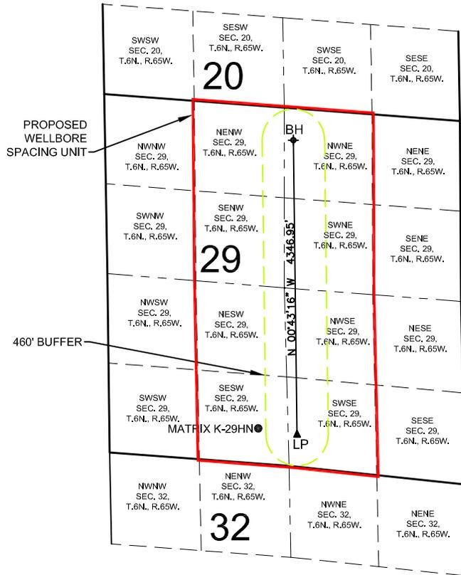
**WELL MATRIX K-29HN TO BE LOCATED 511' FSL AND 2199' FWL, SEC. 29, T6N, R65W**
