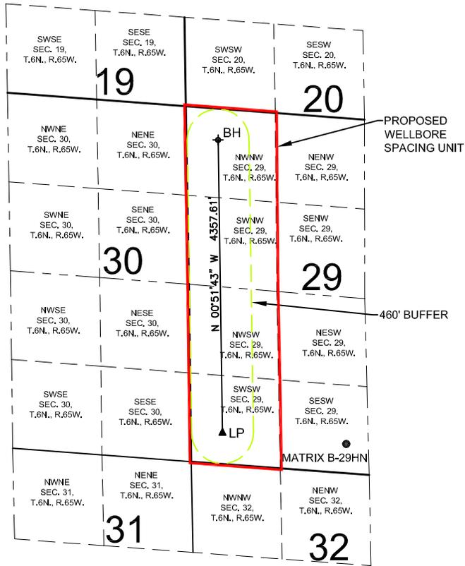
**WELL MATRIX B-29HN TO BE LOCATED 435' FSL AND 2309' FWL, SEC. 29, T6N, R65W**
