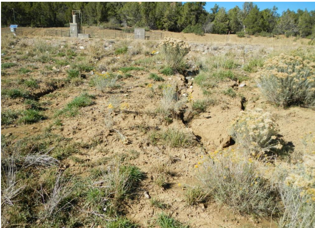
Photo 1. View of rill erosion (approximately 1 foot wide and 1 foot deep) within the southern portion of the interim reclamation area.
