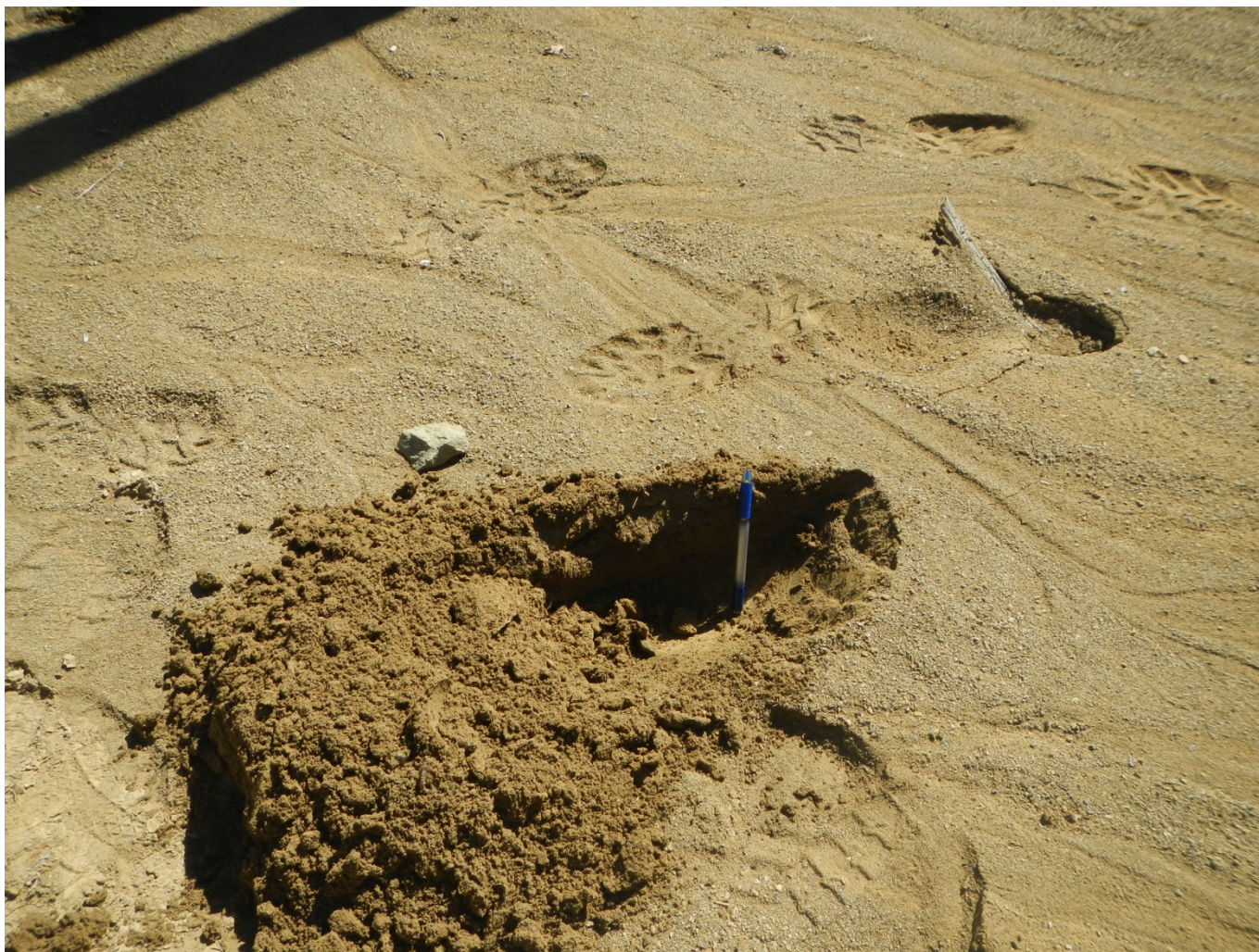
Photo 9. Sediment deposited on the well pad is approximately 6 inches deep in this location.
