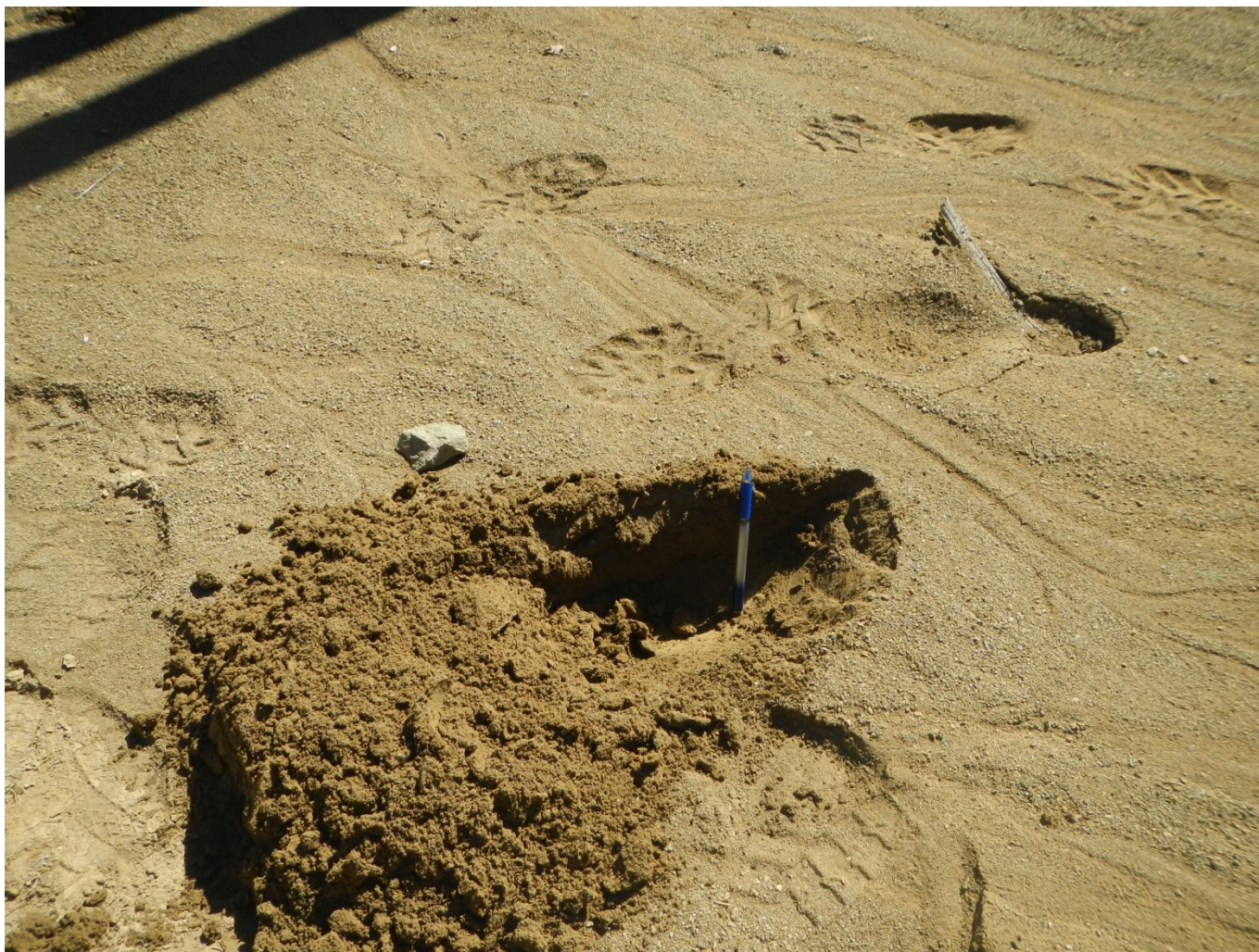
Photo 9. Sediment deposited on the well pad is approximately 6 inches deep.
