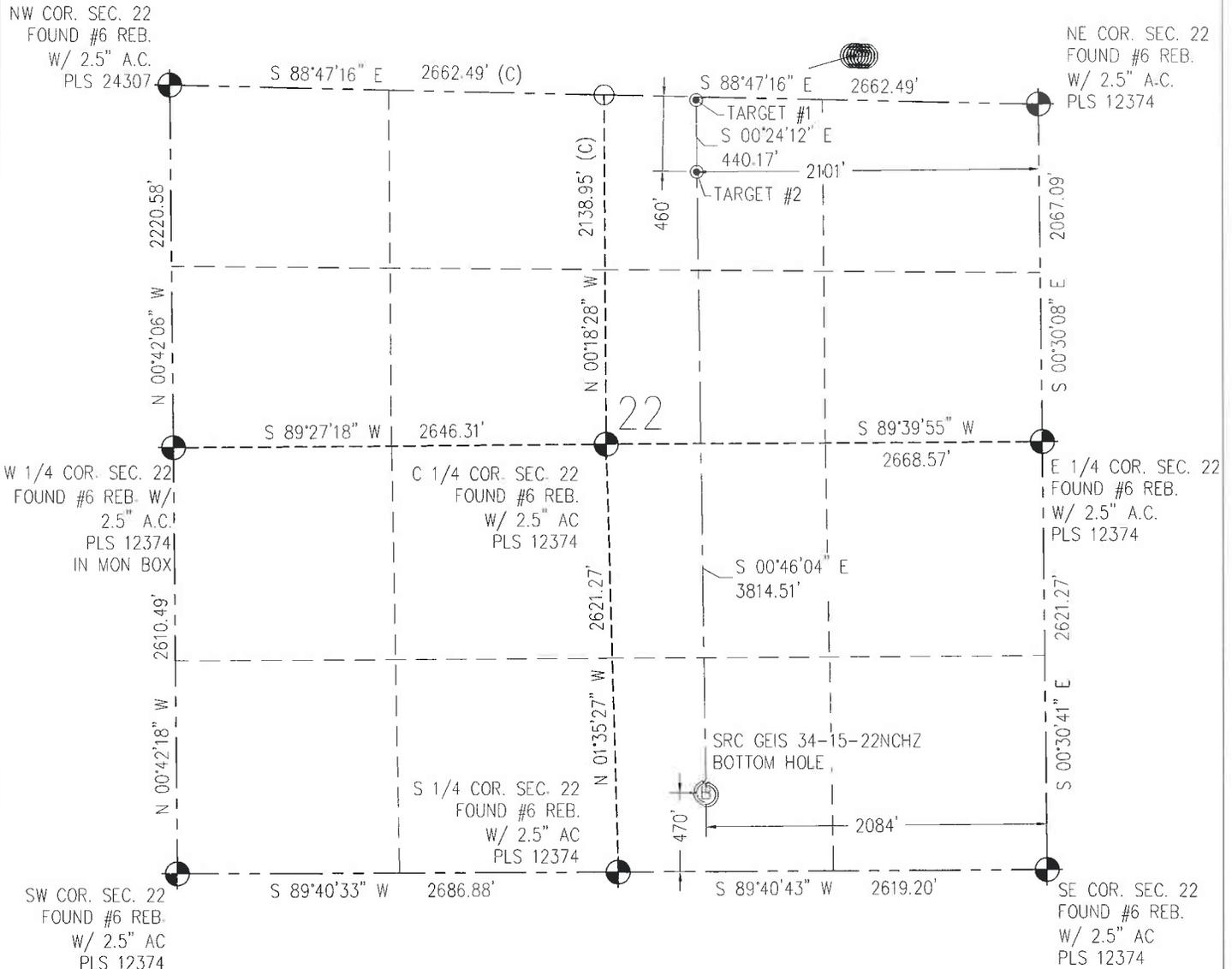
**N** IN ACCORDANCE WITH A REQUEST FROM CRAIG RASMUSON - SYNERGY RESOURCES, BASELINE ENGINEERING CORP. HAS DETERMINED THE LOCATION OF THE SRC GEIS 34-15-22NCHZ TO BE 272' FSL AND 1147' FEL. AS MEASURED AT NINETY (90) DEGREES FROM THE SECTION LINE OF SECTION 15, TOWNSHIP 7 NORTH, RANGE 65 WEST AND THE BOTTOM HOLE LOCATION TO BE 470' FSL AND 2084' FEL OF SECTION 22, TOWNSHIP 7 NORTH, RANGE 65 WEST, 6TH PRINCIPAL MERIDIAN, WELD COUNTY, COLORADO.
