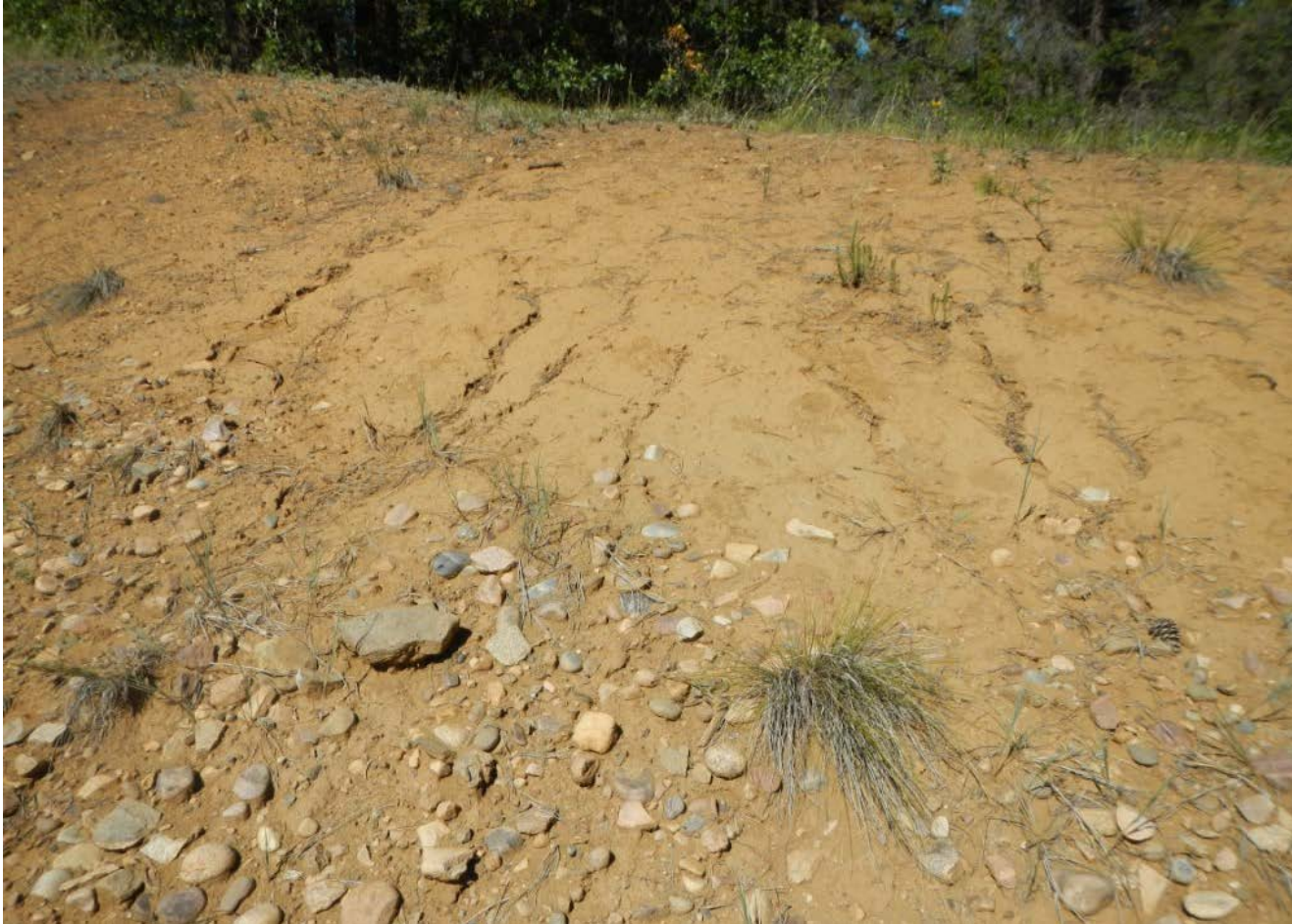
Photo 4. View of rill erosion on the cut slope within the northern portion of the interim reclamation area.
