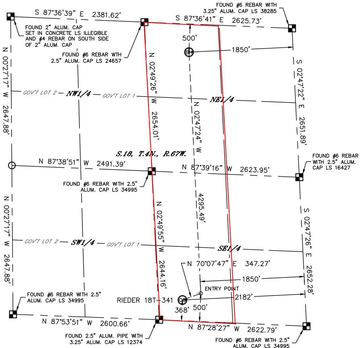
In accordance with a request from Mac Neumann with PDC ENGERY Lat40°, Inc. has determined the surface location of the RIEDER 18T-341 to be 368' from the SOUTH line and 2182' from the EAST line and the bottom hole to be 500' from the NORTH line and 1850' from the EAST line as measured at right angles from the section lines of Section 18, Township 4 North, Range 67 West of the Sixth Principal Meridian, County of Weld, State of Colorado.
