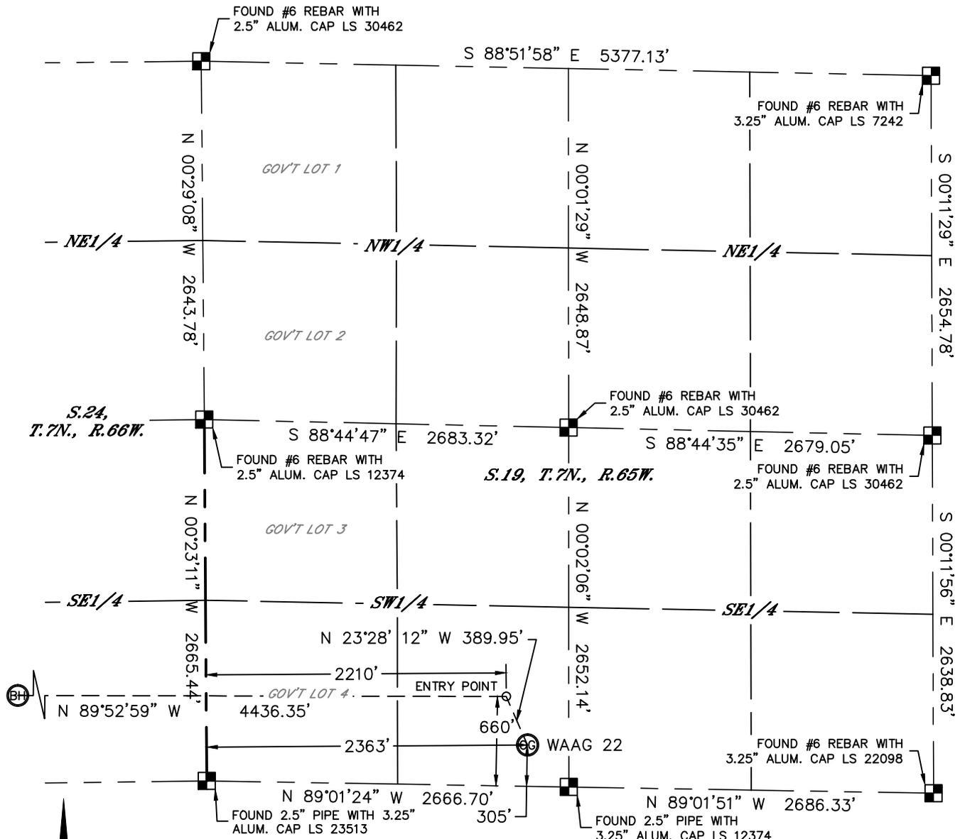
In accordance with a request from Derek Petrie with EXTRACTION OIL & GAS Lat40°, Inc. has determined the surface location of the WAAG 22 to be 305' from the SOUTH line and 2363' from the WEST line of Section 19, Township 7 North, Range 65 West and the bottom hole to be 660' from the SOUTH line and 2226' from the EAST line as measured at right angles from the section lines of Section 24, Township 7 North, Range 66 West of the Sixth Principal Meridian, County of Weld, State of Colorado.
