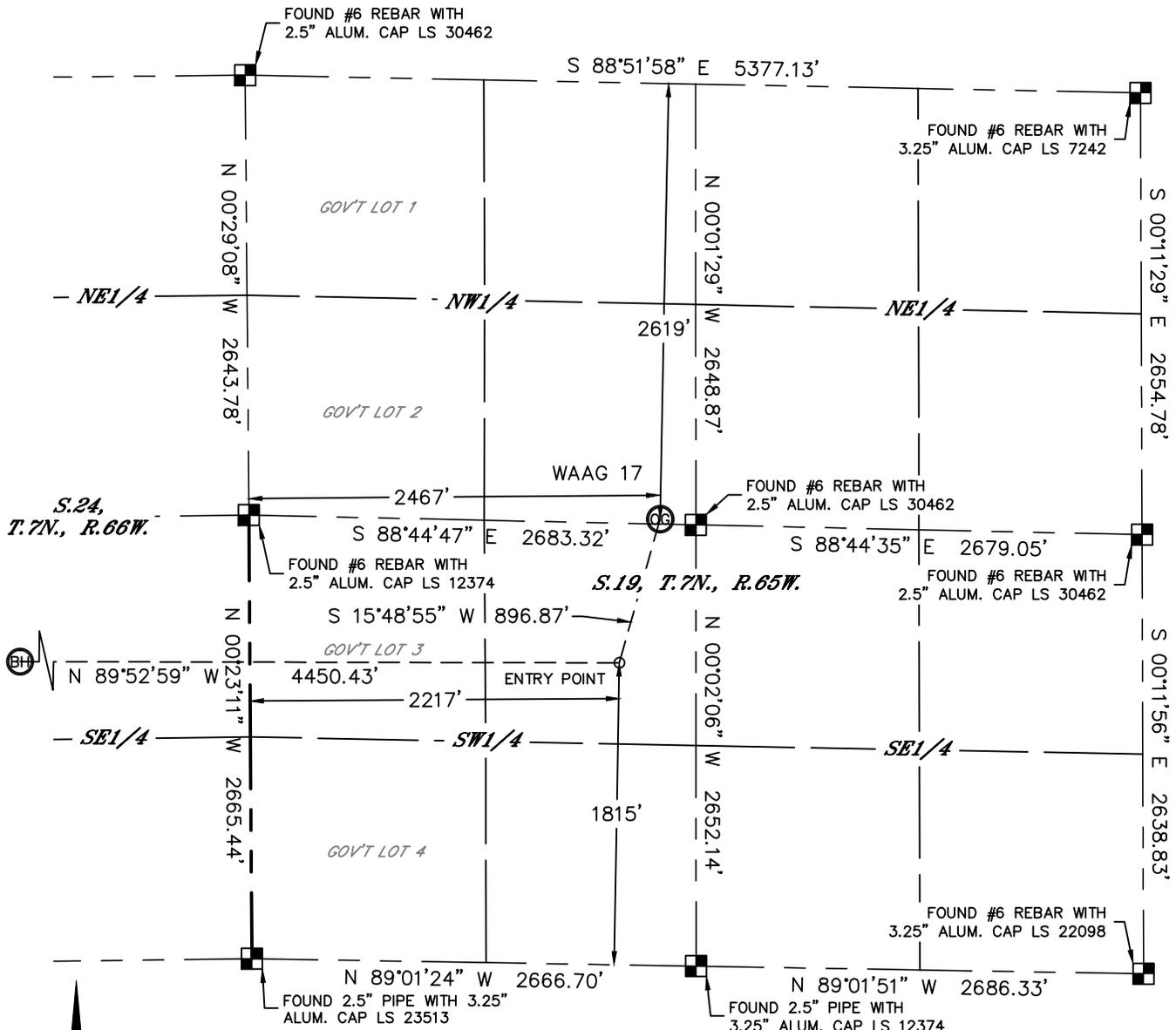
In accordance with a request from Derek Petrie with EXTRACTION OIL & GAS, Lat40°, Inc. has determined the surface location of the WAAG 17 to be 2619' from the NORTH line and 2467' from the WEST line of Section 19, Township 7 North, Range 65 West and the bottom hole to be 1815' from the SOUTH line and 2233' from the EAST line as measured at right angles from the section lines of Section 24, Township 7 North, Range 66 West of the Sixth Principal Meridian, County of Weld, State of Colorado.
