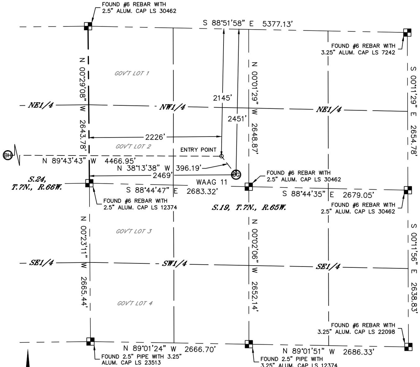
In accordance with a request from Derek Petrie with EXTRACTION OIL & GAS Lat40°, Inc. has determined the surface location of the WAAG 11 to be 2451' from the NORTH line and 2469' from the WEST line of Section 19, Township 7 North, Range 65 West and the bottom hole to be 2145' from the NORTH line and 2240' from the EAST line as measured at right angles from the section lines of Section 24, Township 7 North, Range 66 West of the Sixth Principal Meridian, County of Weld, State of Colorado.
