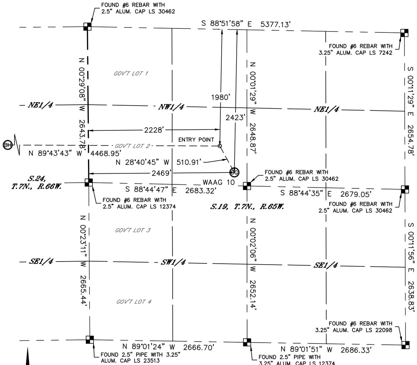
In accordance with a request from Derek Petrie with EXTRACTION OIL & GAS Lat40°, Inc. has determined the surface location of the WAAG 10 to be 2423' from the NORTH line and 2469' from the WEST line of Section 19, Township 7 North, Range 65 West and the bottom hole to be 1980' from the NORTH line and 2241' from the EAST line as measured at right angles from the section lines of Section 24, Township 7 North, Range 66 West of the Sixth Principal Meridian, County of Weld, State of Colorado.
