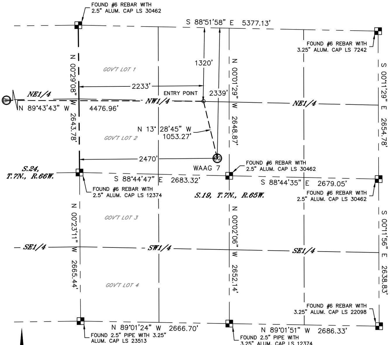
In accordance with a request from Derek Petrie with EXTRACTION OIL & GAS Lat40°, Inc. has determined the surface location of the WAAG 7 to be 2339' from the NORTH line and 2470' from the WEST line of Section 19, Township 7 North, Range 65 West and the bottom hole to be 1320' from the NORTH line and 2244' from the EAST line as measured at right angles from the section lines of Section 24, Township 7 North, Range 66 West of the Sixth Principal Meridian, County of Weld, State of Colorado.
