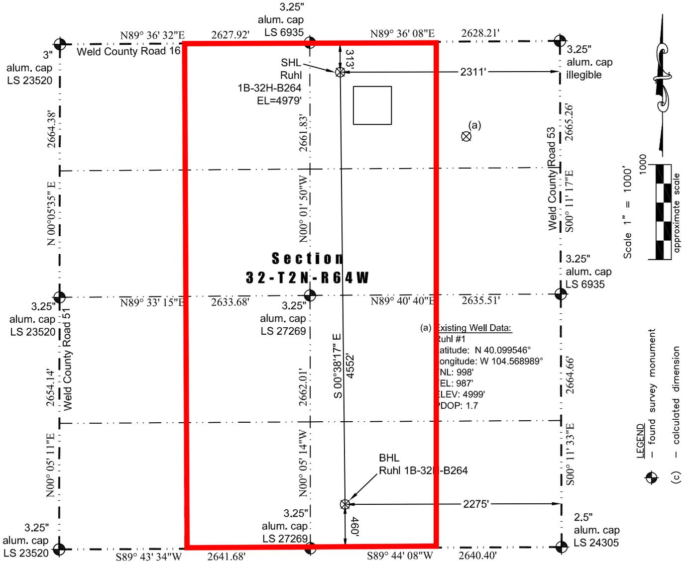
In accordance with a request from Jay Knutson of EnCana Oil & Gas (USA) Inc., Washburn Land Surveying, LLC has determined the location of the **Ruhl 1B-32H-B264** well site to be SHL: 313' FNL and 2311' FEL, (BHL: 460' FSL and 2275' FEL), as measured at ninety (90) degrees from the section lines of Section 32, Township 2 North, Range 64 West of the 6th Principal Meridian, Weld County Colorado.
