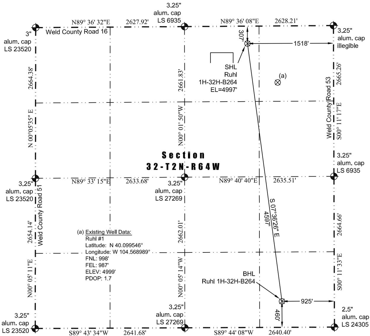
In accordance with a request from Jay Knutson of EnCana Oil & Gas (USA) Inc., Washburn Land Surveying, LLC has determined the location of the **Ruhl 1H-32H-B264** well site to be SHL: 307' FNL and 1518' FEL, (BHL: 460' FSL and 925' FEL), as measured at ninety (90) degrees from the section lines of Section 32, Township 2 North, Range 64 West of the 6th Principal Meridian, Weld County Colorado.
