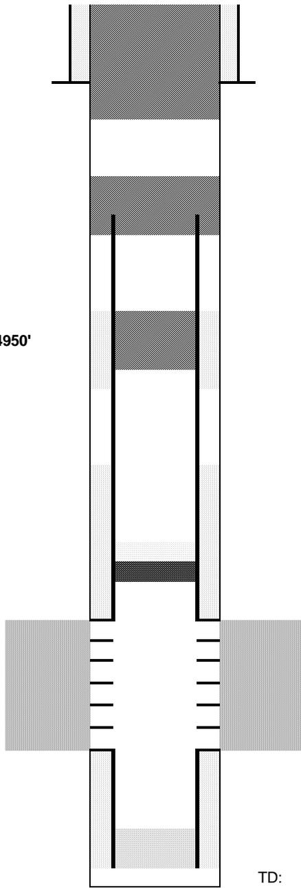
Cut surface casing off 6'-8' below surface.
