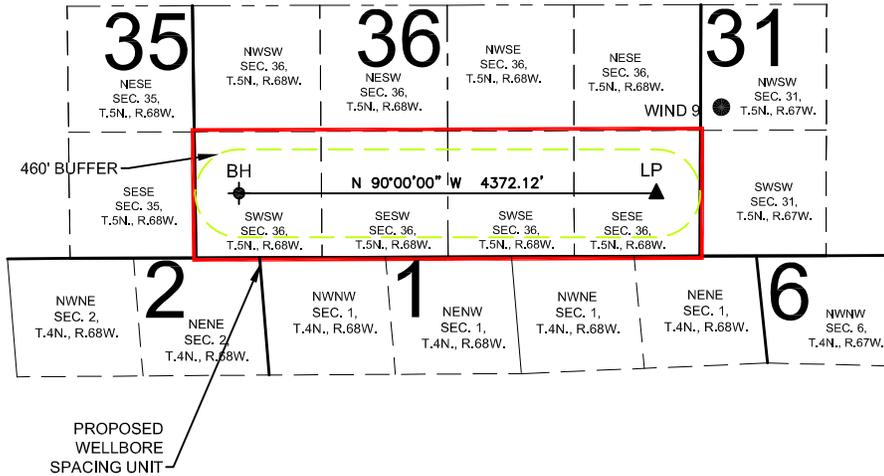
WELL **WIND 9** TO BE LOCATED 1602' FSL AND 240' FWL, SEC. 31, T5N, R67W
