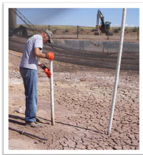
Figure 1: Sampling the southwest corner of the reserve pit using a push core sampler.
