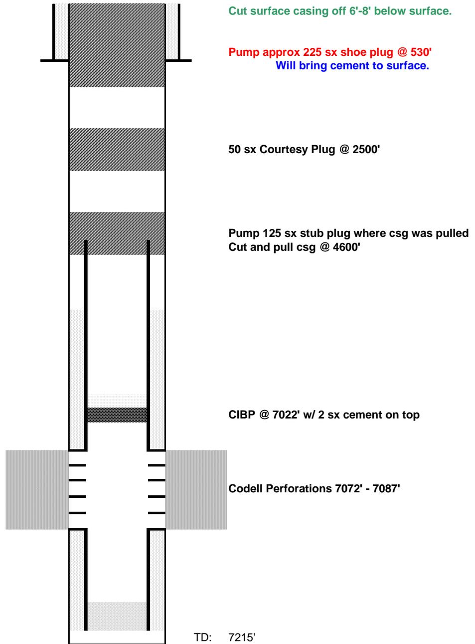
Cut surface casing off 6'-8' below surface.
