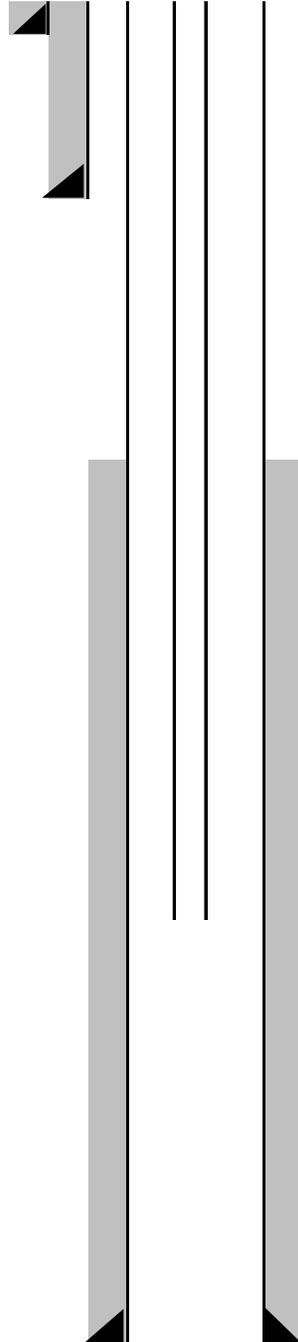
Conductor 26" Hole 18" casing/liner 44' W/ 16 Sks cmt
