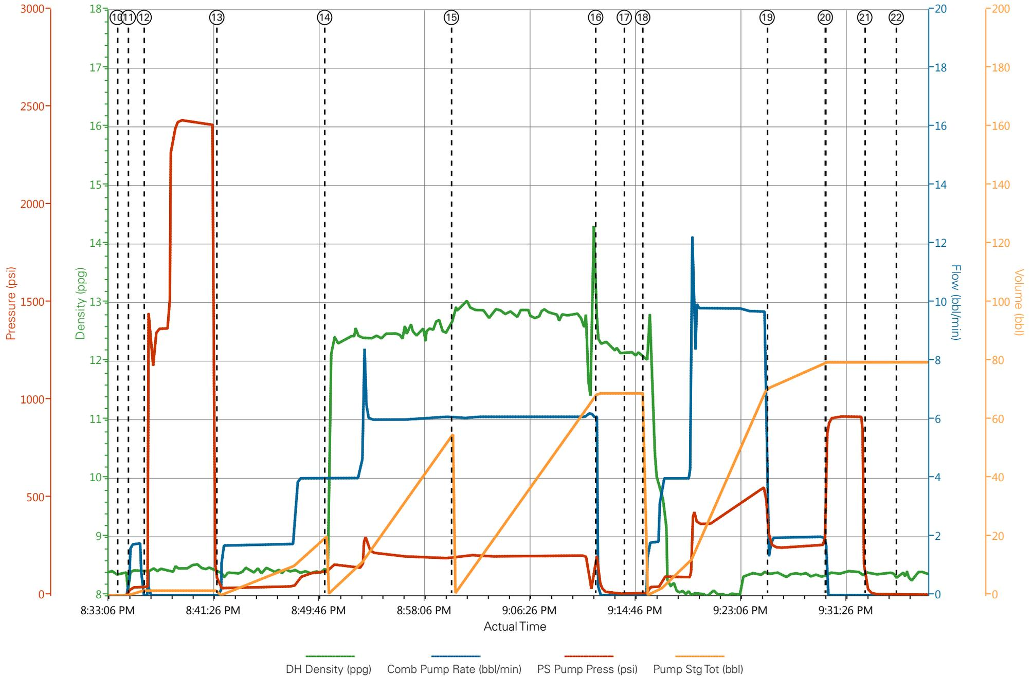
DH Density (ppg) Comb Pump Rate (bbl/min) PS Pump Press (psi) Pump Stg Tot (bbl)
