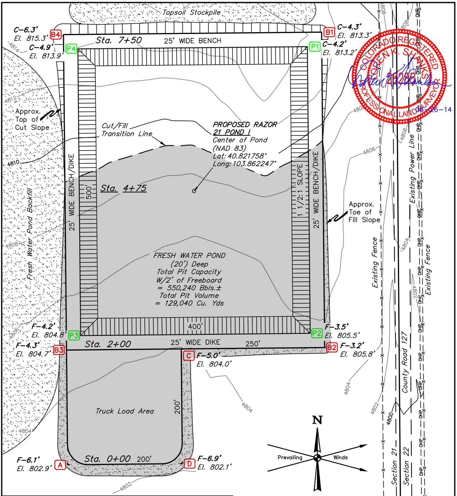
FINISHED GRADE ELEVATION AT POND BENCH = 4809.0'
