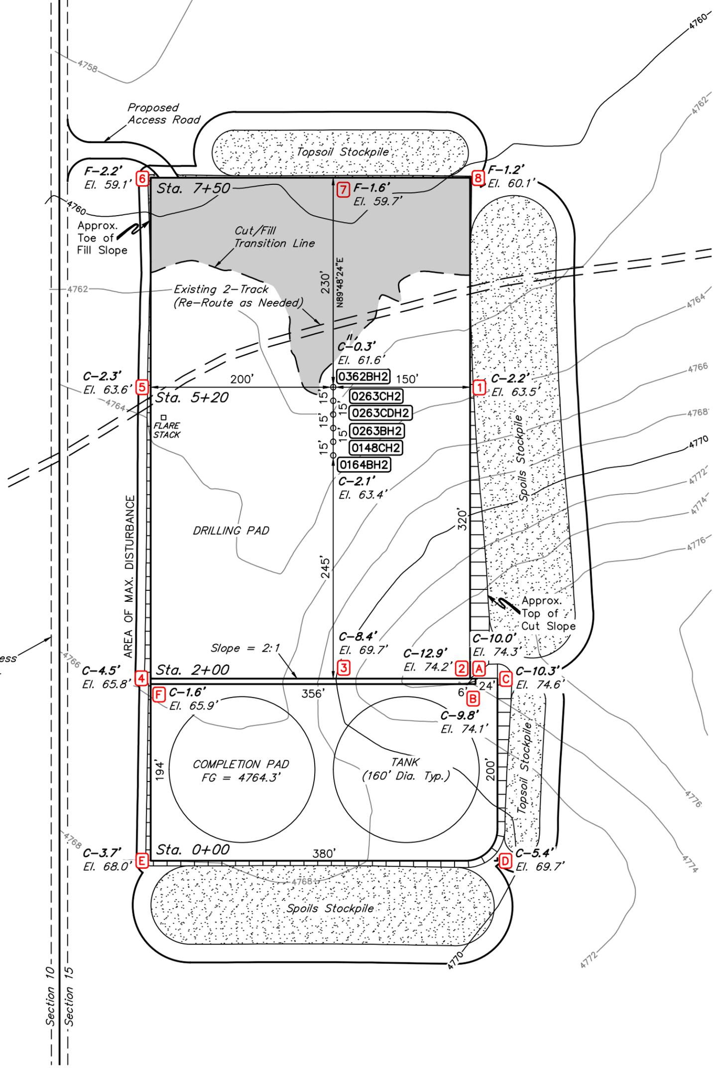
**DRILLING PAD FINISHED GRADE ELEVATION = 4761.3'**
