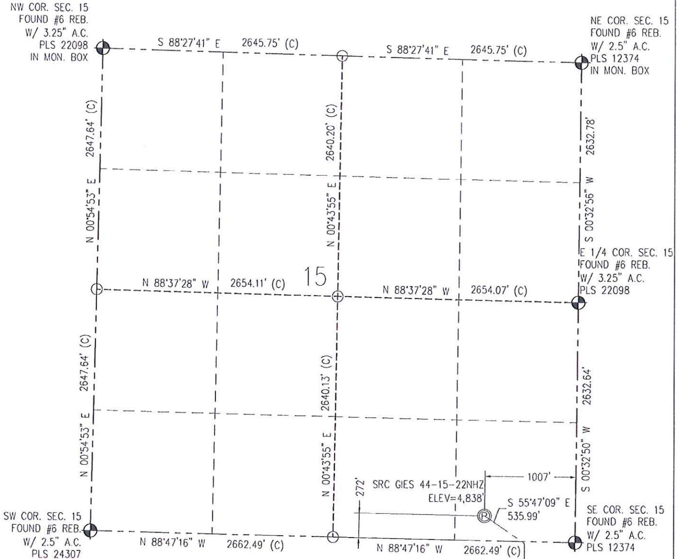
IN ACCORDANCE WITH A REQUEST FROM CRAIG RASMUSON - SYNERGY RESOURCES, BASELINE ENGINEERING CORP. HAS DETERMINED THE LOCATION OF THE SRC GIES 44-15-22NHZ TO BE 272' FSL AND 1007' FEL, AS MEASURED AT NINETY (90) DEGREES FROM THE SECTION LINE OF SECTION 15, TOWNSHIP 7 NORTH, RANGE 65 WEST AND THE BOTTOM HOLE LOCATION TO BE 470' FSL AND 544' FEL OF SECTION 22, TOWNSHIP 7 NORTH, RANGE 65 WEST, 6TH PRINCIPAL MERIDIAN, WELD COUNTY, COLORADO.
