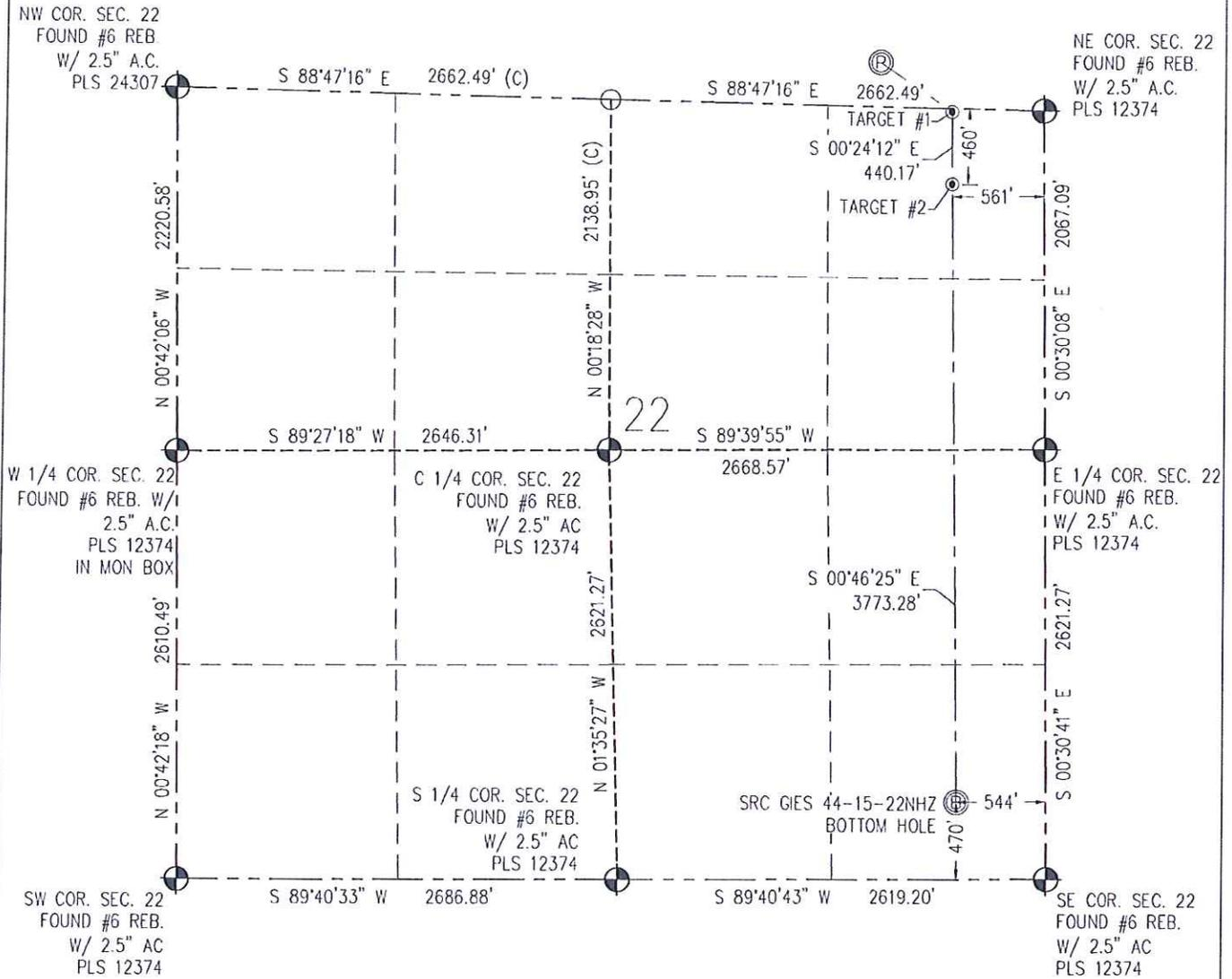
IN ACCORDANCE WITH A REQUEST FROM CRAIG RASMUSON - SYNERGY RESOURCES, BASELINE ENGINEERING CORP. HAS DETERMINED THE LOCATION OF THE SRC GIES 44-15-22NHZ TO BE 272' FSL AND 1007' FEL, AS MEASURED AT NINETY (90) DEGREES FROM THE SECTION LINE OF SECTION 15, TOWNSHIP 7 NORTH, RANGE 65 WEST AND THE BOTTOM HOLE LOCATION TO BE 470' FSL AND 544' FEL OF SECTION 22, TOWNSHIP 7 NORTH, RANGE 65 WEST, 6TH PRINCIPAL MERIDIAN, WELD COUNTY, COLORADO.
