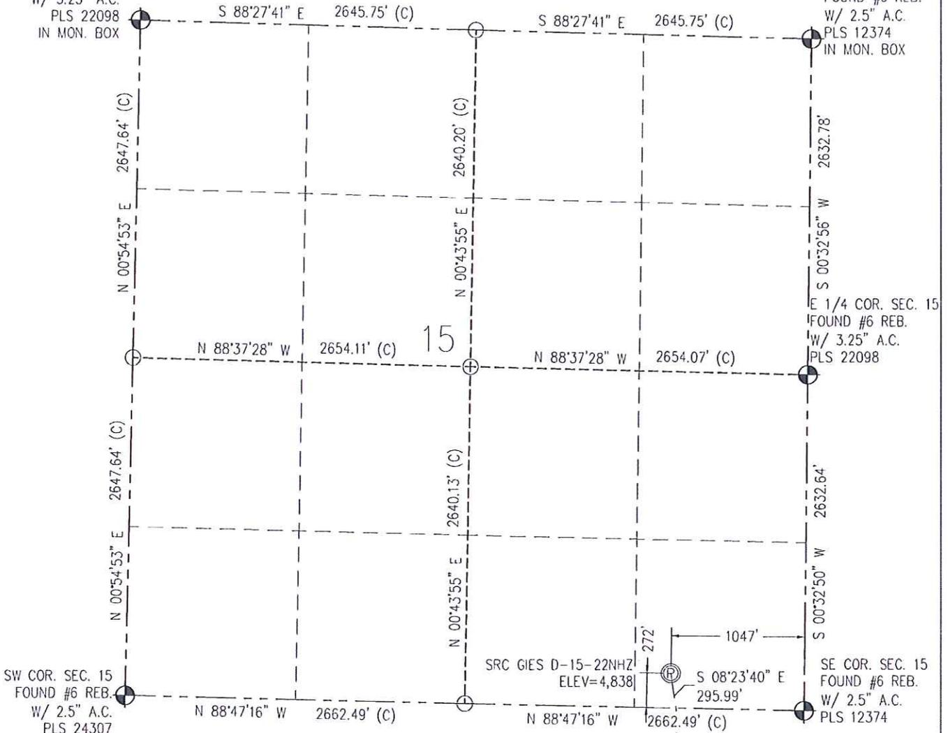
IN ACCORDANCE WITH A REQUEST FROM CRAIG RASMUSON - SYNERGY RESOURCES, BASELINE ENGINEERING CORP. HAS DETERMINED THE LOCATION OF THE SRC GIES D-15-22NHZ TO BE 272' FSL AND 1047' FEL, AS MEASURED AT NINETY (90) DEGREES FROM THE SECTION LINE OF SECTION 15, TOWNSHIP 7 NORTH, RANGE 65 WEST AND THE BOTTOM HOLE LOCATION TO BE 470' FSL AND 984' FEL OF SECTION 22, TOWNSHIP 7 NORTH, RANGE 65 WEST, 6TH PRINCIPAL MERIDIAN, WELD COUNTY, COLORADO.
