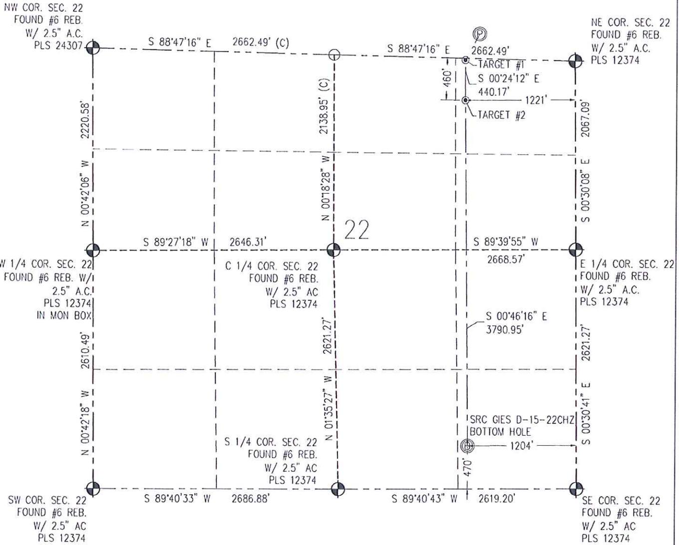
IN ACCORDANCE WITH A REQUEST FROM CRAIG RASMUSON - SYNERGY RESOURCES, BASELINE ENGINEERING CORP. HAS DETERMINED THE LOCATION OF THE SRC GIES D-15-22CHZ TO BE 272' FSL AND 1067' FEL, AS MEASURED AT NINETY (90) DEGREES FROM THE SECTION LINE OF SECTION 15, TOWNSHIP 7 NORTH, RANGE 65 WEST AND THE BOTTOM HOLE LOCATION TO BE 470' FSL AND 1204' FEL OF SECTION 22, TOWNSHIP 7 NORTH, RANGE 65 WEST, 6TH PRINCIPAL MERIDIAN, WELD COUNTY, COLORADO
