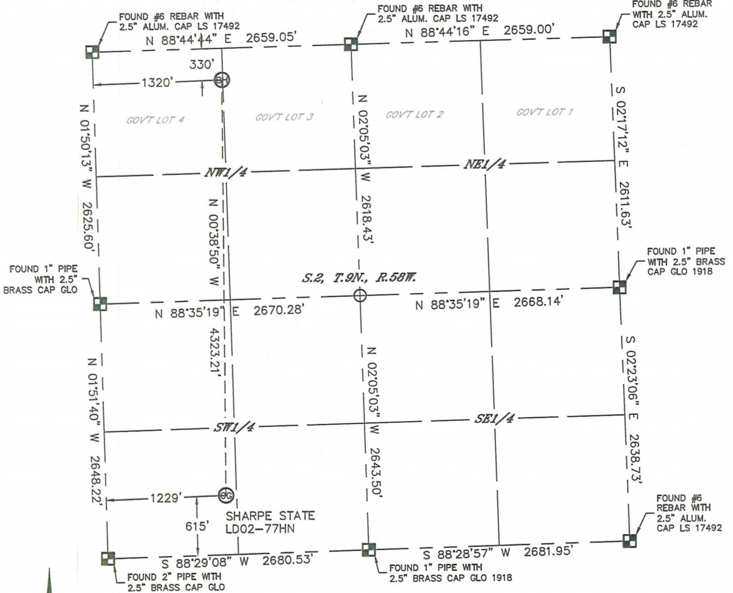
In accordance with a request from Cody Ball with Noble Energy Inc. Lat40°, Inc. has determined the surface location of the SHARPE STATE LD02-77HN to be 615' from the SOUTH line and 1229' from the WEST line and the bottom hole to be 330' from the NORTH line and 1320' from the WEST line as measured at right angles from the section lines of Section 2, Township 9 North, Range 58 West of the Sixth Principal Meridian, County of Weld, State of Colorado.
