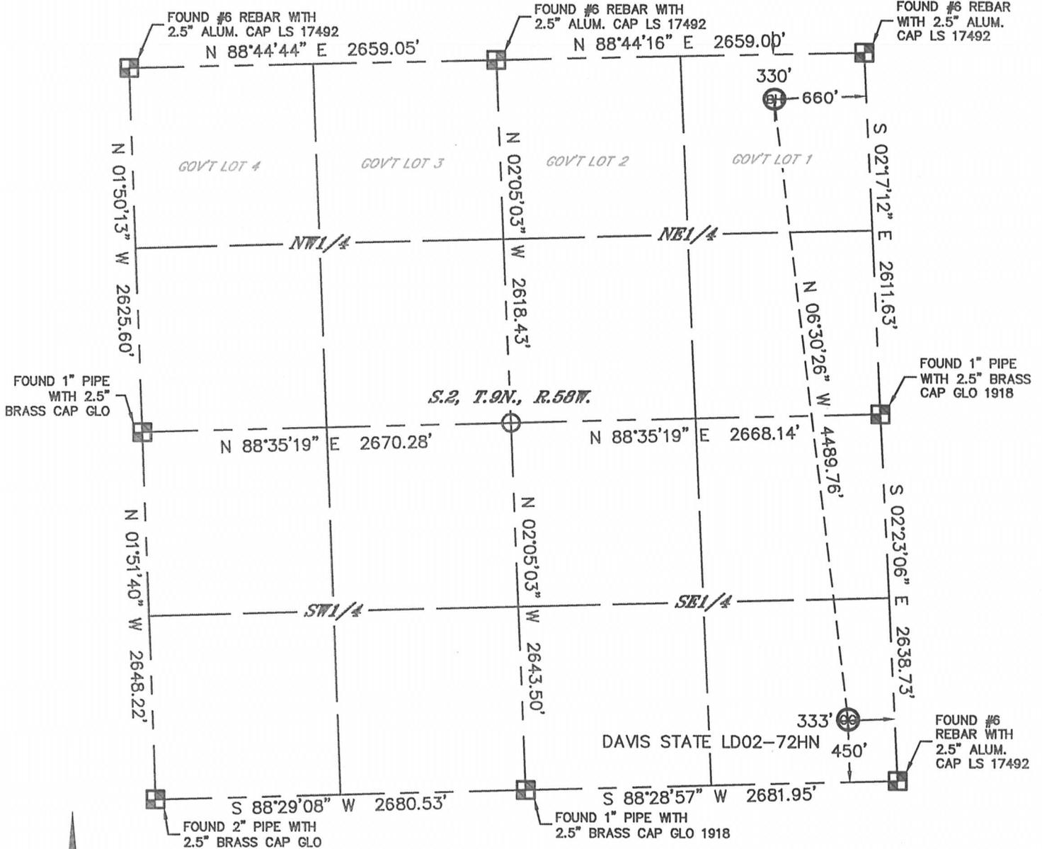
In accordance with a request from Cody Ball with Noble Energy Inc. Lat40°, Inc. has determined the surface location of the DAVIS STATE LD02-72HN to be 450' from the SOUTH line and 333' from the EAST line and the bottom hole to be 330' from the NORTH line and 660' from the EAST line as measured at right angles from the section lines of Section 2, Township 9 North, Range 58 West of the Sixth Principal Meridian, County of Weld, State of Colorado.
