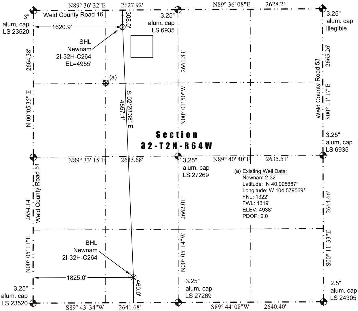
In accordance with a request from Jay Knutson of EnCana Oil & Gas (USA) Inc., JR Land Surveying, LLC has determined the location of the **Newnam 2I-32H-C264** well site to be SHL: 308.0' FNL and 1620.9 FWL, (BHL: 460.0' FSL and 1825.0' FWL), as measured at ninety (90) degrees from the section lines of Section 32, Township 2 North, Range 64 West of the 6th Principal Meridian, Weld County Colorado.
