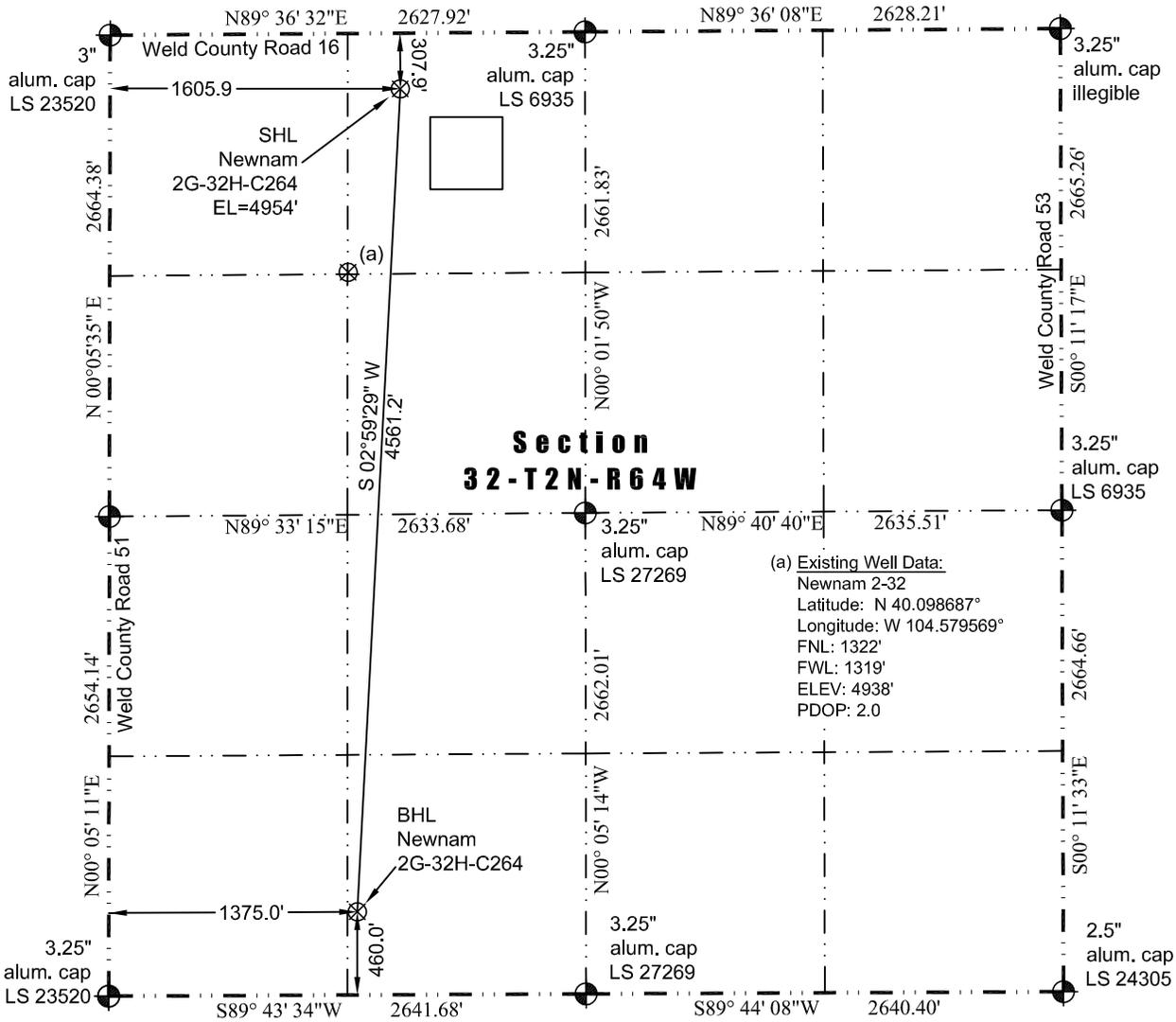
In accordance with a request from Jay Knutson of EnCana Oil & Gas (USA) Inc., JR Land Surveying, LLC has determined the location of the **Newnam 2G-32H-C264** well site to be SHL: 307.9' FNL and 1605.9' FWL, (BHL: 460.0' FSL and 1375.0' FWL), as measured at ninety (90) degrees from the section lines of Section 32, Township 2 North, Range 64 West of the 6th Principal Meridian, Weld County Colorado.
