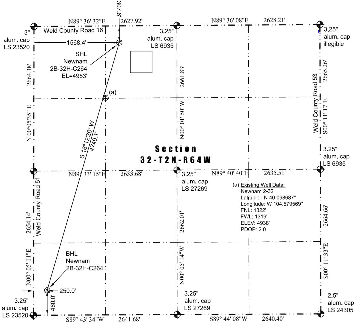
In accordance with a request from Jay Knutson of EnCana Oil & Gas (USA) Inc., JR Land Surveying, LLC has determined the location of the **Newnam 2B-32H-C264** well site to be SHL: 307.6' FNL and 1568.4' FWL, (BHL: 460.0' FSL and 250.0' FWL), as measured at ninety (90) degrees from the section lines of Section 32, Township 2 North, Range 64 West of the 6th Principal Meridian, Weld County Colorado.
