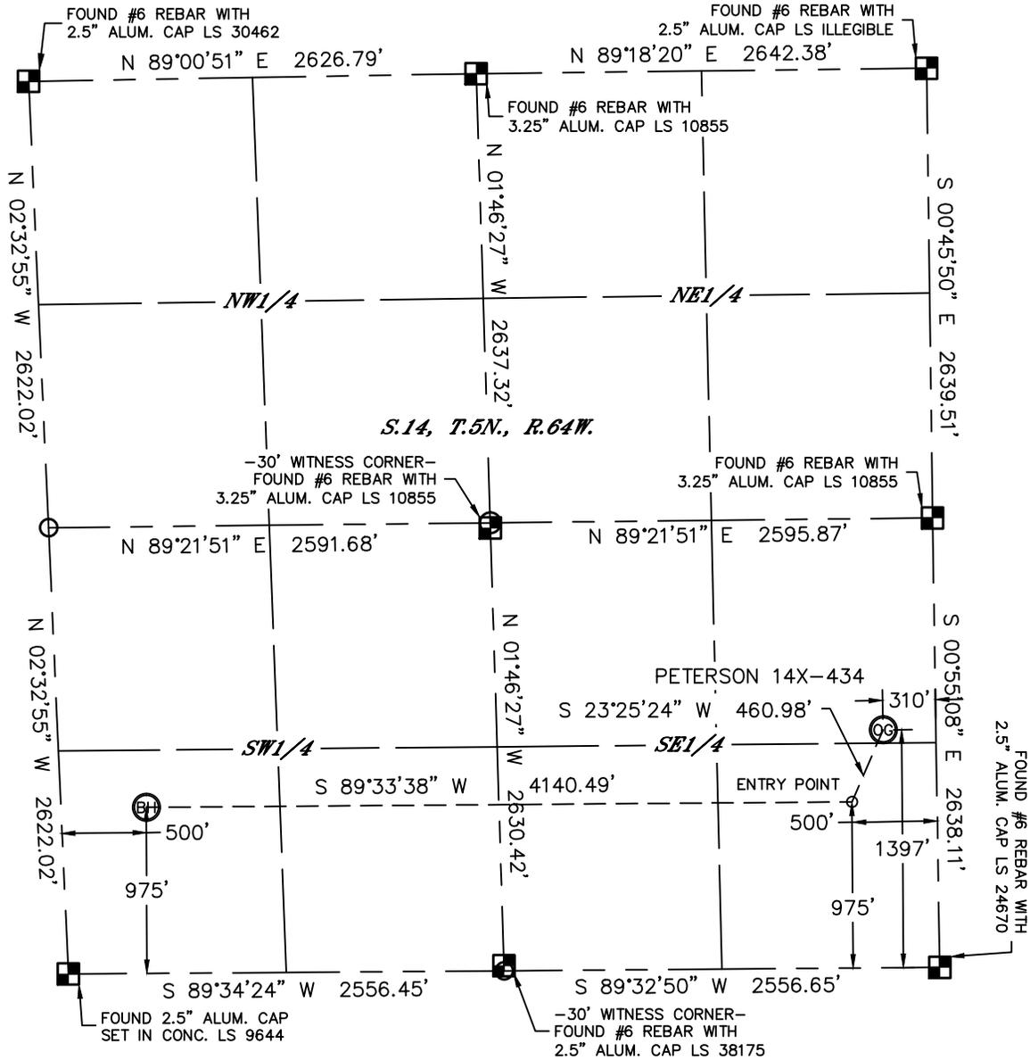
In accordance with a request from Al Bragg with PDC ENERGY Lat40°, Inc. has determined the surface location of the PETERSON 14X-434 to be 1397' from the SOUTH line and 310' from the EAST line and the bottom hole to be 975' from the SOUTH line and 500' from the WEST line as measured at right angles from the section lines of Section 14, Township 5 North, Range 64 West of the Sixth Principal Meridian, County of Weld, State of Colorado.
