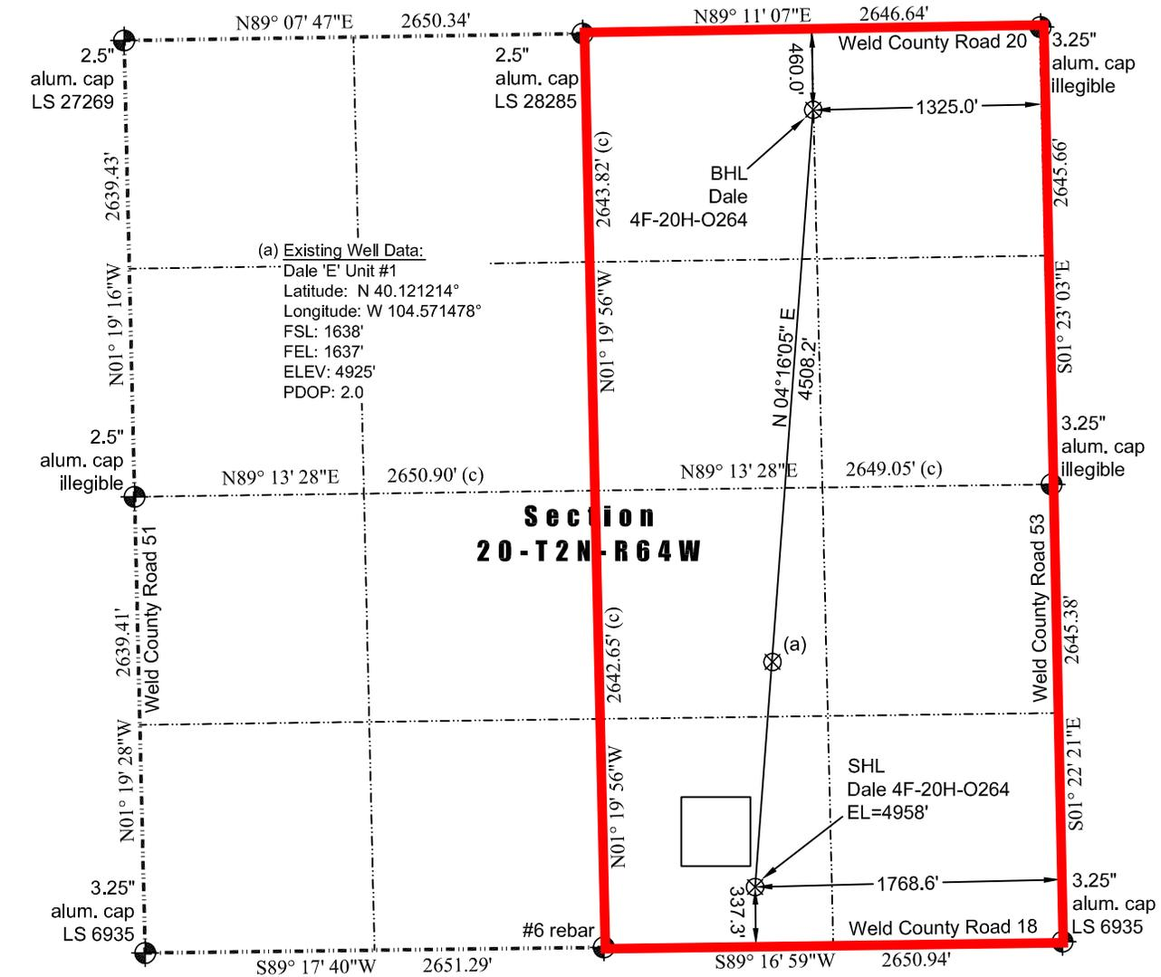
In accordance with a request from Jay Knutson of EnCana Oil & Gas (USA) Inc., JR Land Surveying, LLC has determined the location of the **Dale 4F-20H-O264** well site to be SHL: 337.3' FSL and 1768.6' FEL, (BHL: 460.0' FNL and 1325.0' FEL), as measured at ninety (90) degrees from the section lines of Section 20, Township 2 North, Range 64 West of the 6th Principal Meridian, Weld County Colorado.
