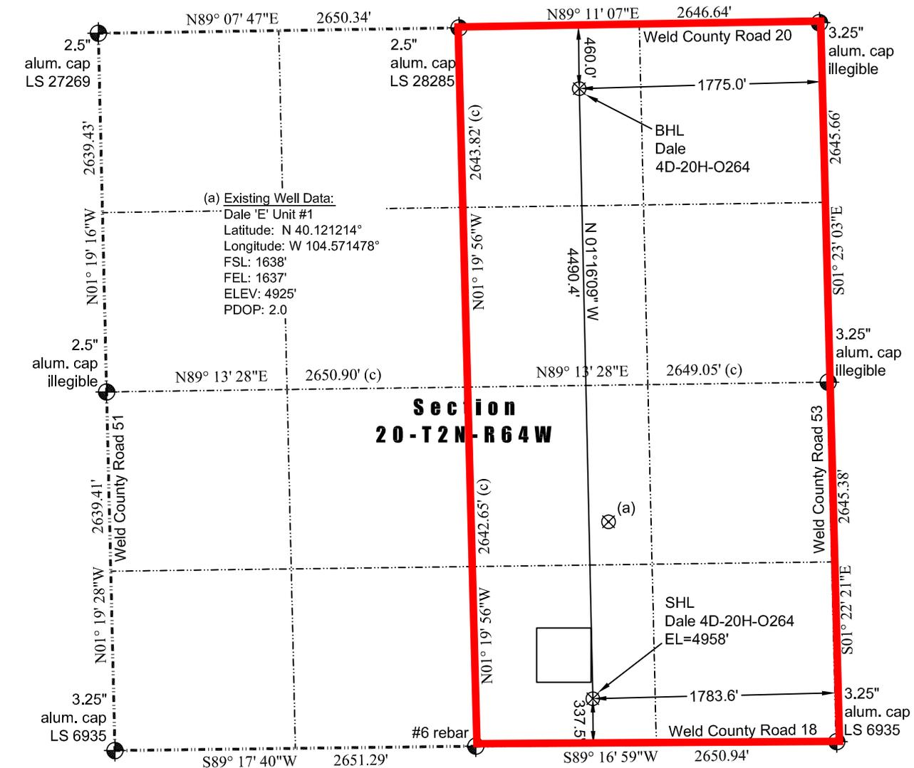
In accordance with a request from Jay Knutson of EnCana Oil & Gas (USA) Inc., JR Land Surveying, LLC has determined the location of the **Dale 4D-20H-O264** well site to be SHL: 337.5' FSL and 1783.6' FEL, (BHL: 460.0' FNL and 1775.0' FEL), as measured at ninety (90) degrees from the section lines of Section 20, Township 2 North, Range 64 West of the 6th Principal Meridian, Weld County Colorado.
