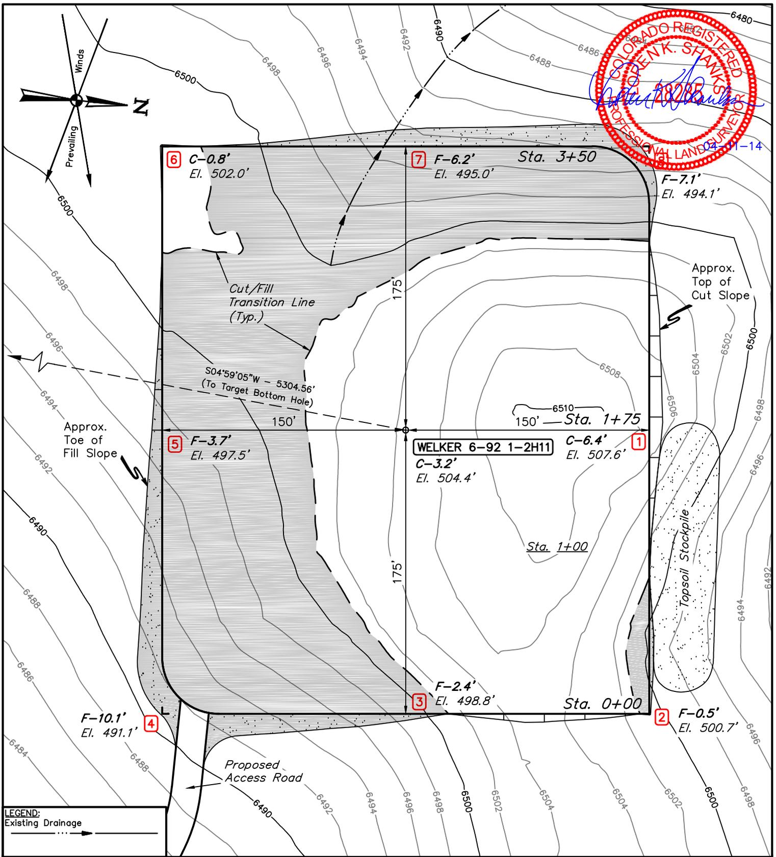
UNGRADED GROUND ELEV. AT LOC. STAKE = **6504.4'** FINISHED GRADE ELEV. AT LOC. STAKE = **6501.2'**
