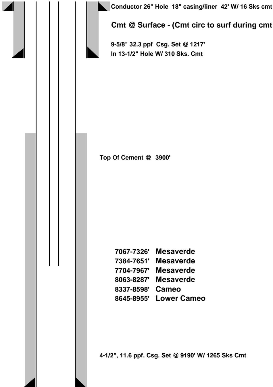
Conductor 26" Hole 18" casing/liner 42' W/ 16 Sks cmt
