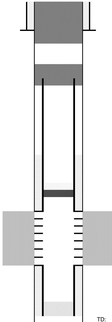
Cut surface casing off 6'-8' below surface.
