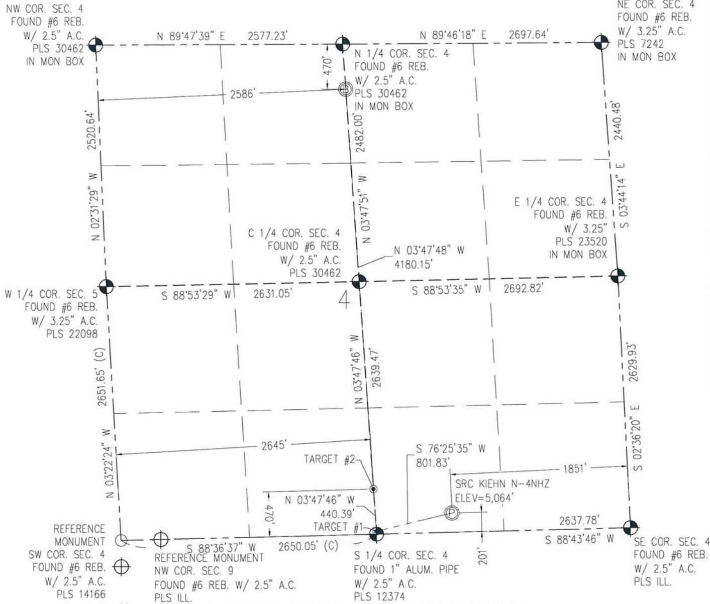
IN ACCORDANCE WITH A REQUEST FROM CRAIG RASMUSON - SYNERGY RESOURCES, BASELINE ENGINEERING CORP. HAS DETERMINED THE LOCATION OF THE SRC KIEHN N-4NHZ TO BE 201' FSL AND 1851' FEL, AS MEASURED AT NINETY (90) DEGREES FROM THE SECTION LINE OF SECTION 4, TOWNSHIP 4 NORTH, RANGE 68 WEST AND THE BOTTOM HOLE LOCATION TO BE 470' FNL AND 2586' FWL OF SECTION 4, TOWNSHIP 4 NORTH, RANGE 68 WEST, 6TH PRINCIPAL MERIDIAN, WELD COUNTY, COLORADO.
