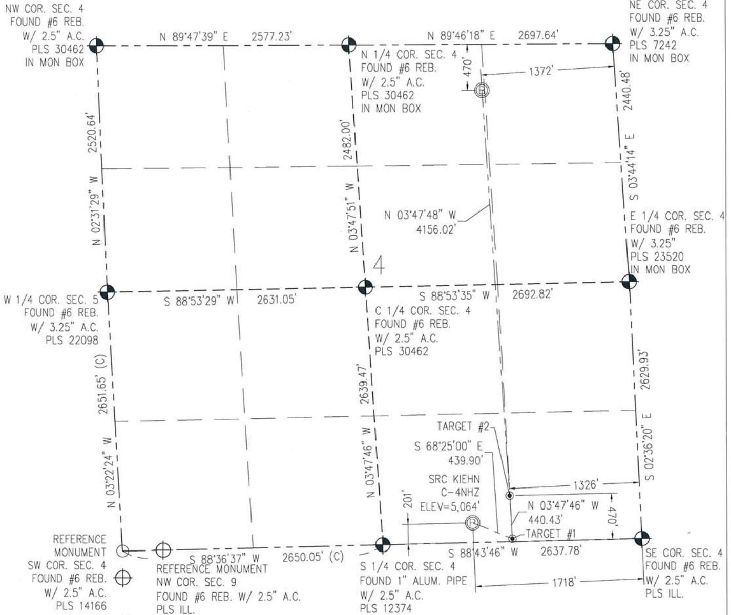
IN ACCORDANCE WITH A REQUEST FROM CRAIG RASMUSON - SYNERGY RESOURCES, BASELINE ENGINEERING CORP. HAS DETERMINED THE LOCATION OF THE SRC KIEHN C-4NHZ TO BE 201' FSL AND 1718' FEL, AS MEASURED AT NINETY (90) DEGREES FROM THE SECTION LINE OF SECTION 4, TOWNSHIP 4 NORTH, RANGE 68 WEST AND THE BOTTOM HOLE LOCATION TO BE 470' FNL AND 1372' FEL OF SECTION 4, TOWNSHIP 4 NORTH, RANGE 68 WEST, 6TH PRINCIPAL MERIDIAN, WELD COUNTY, COLORADO.
