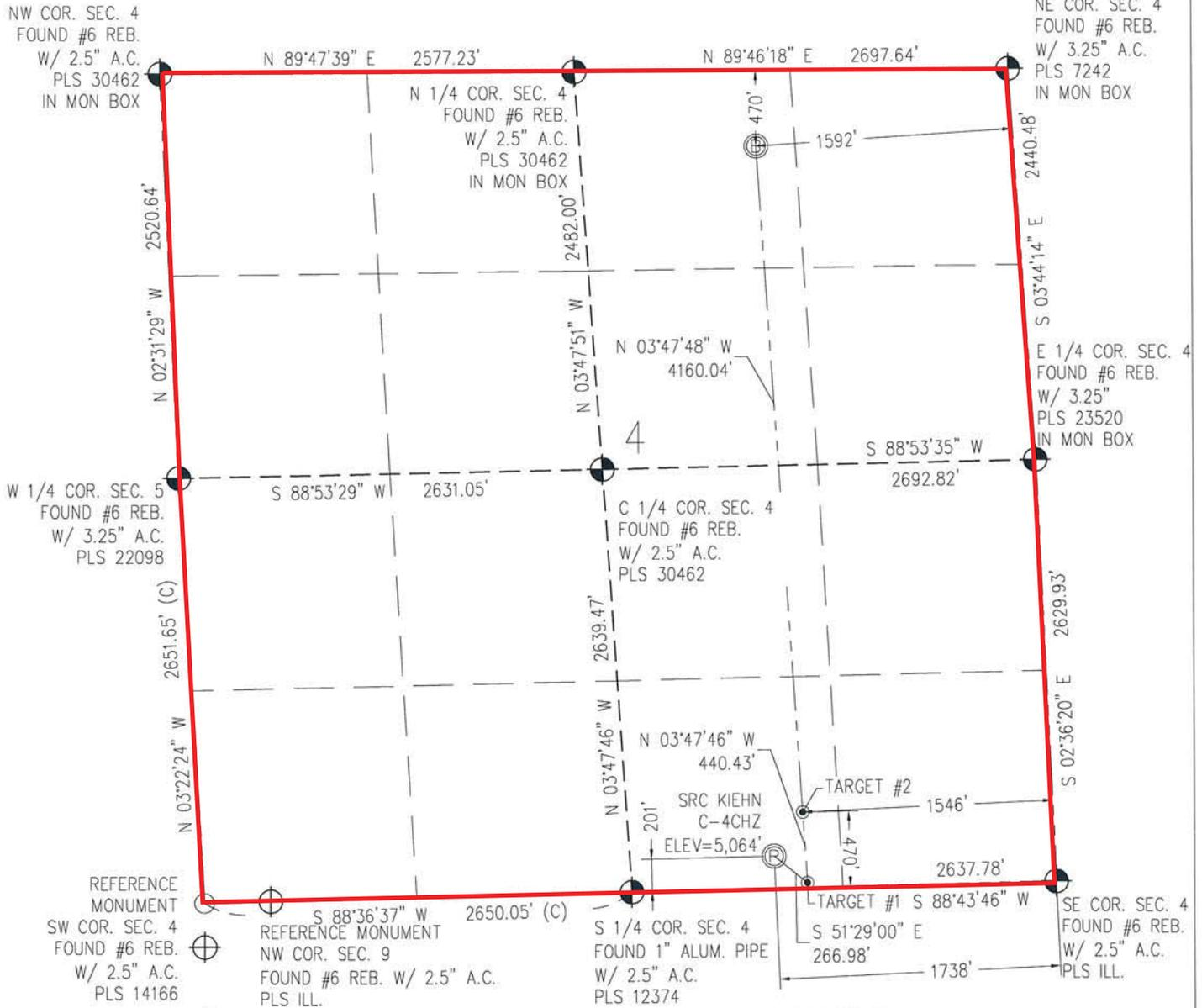
IN ACCORDANCE WITH A REQUEST FROM CRAIG RASMUSON - SYNERGY RESOURCES, BASELINE ENGINEERING CORP. HAS DETERMINED THE LOCATION OF THE SRC KIEHN C-4CHZ TO BE 201' FSL AND 1738' FEL, AS MEASURED AT NINETY (90) DEGREES FROM THE SECTION LINE OF SECTION 4, TOWNSHIP 4 NORTH, RANGE 68 WEST AND THE BOTTOM HOLE LOCATION TO BE 470' FNL AND 1592' FEL OF SECTION 4, TOWNSHIP 4 NORTH, RANGE 68 WEST, 6TH PRINCIPAL MERIDIAN, WELD COUNTY, COLORADO.
