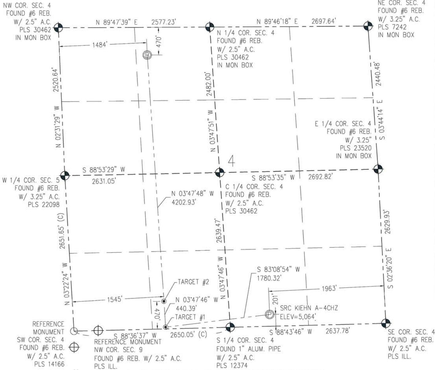
IN ACCORDANCE WITH A REQUEST FROM CRAIG RASMUSON - SYNERGY RESOURCES, BASELINE ENGINEERING CORP. HAS DETERMINED THE LOCATION OF THE SRC KIEHN A-4CHZ TO BE 201' FSL AND 1963' FEL, AS MEASURED AT NINETY (90) DEGREES FROM THE SECTION LINE OF SECTION 4, TOWNSHIP 4 NORTH, RANGE 68 WEST AND THE BOTTOM HOLE LOCATION TO BE 470' FNL AND 1484' FWL OF SECTION 4, TOWNSHIP 4 NORTH, RANGE 68 WEST, 6TH PRINCIPAL MERIDIAN, WELD COUNTY, COLORADO.
