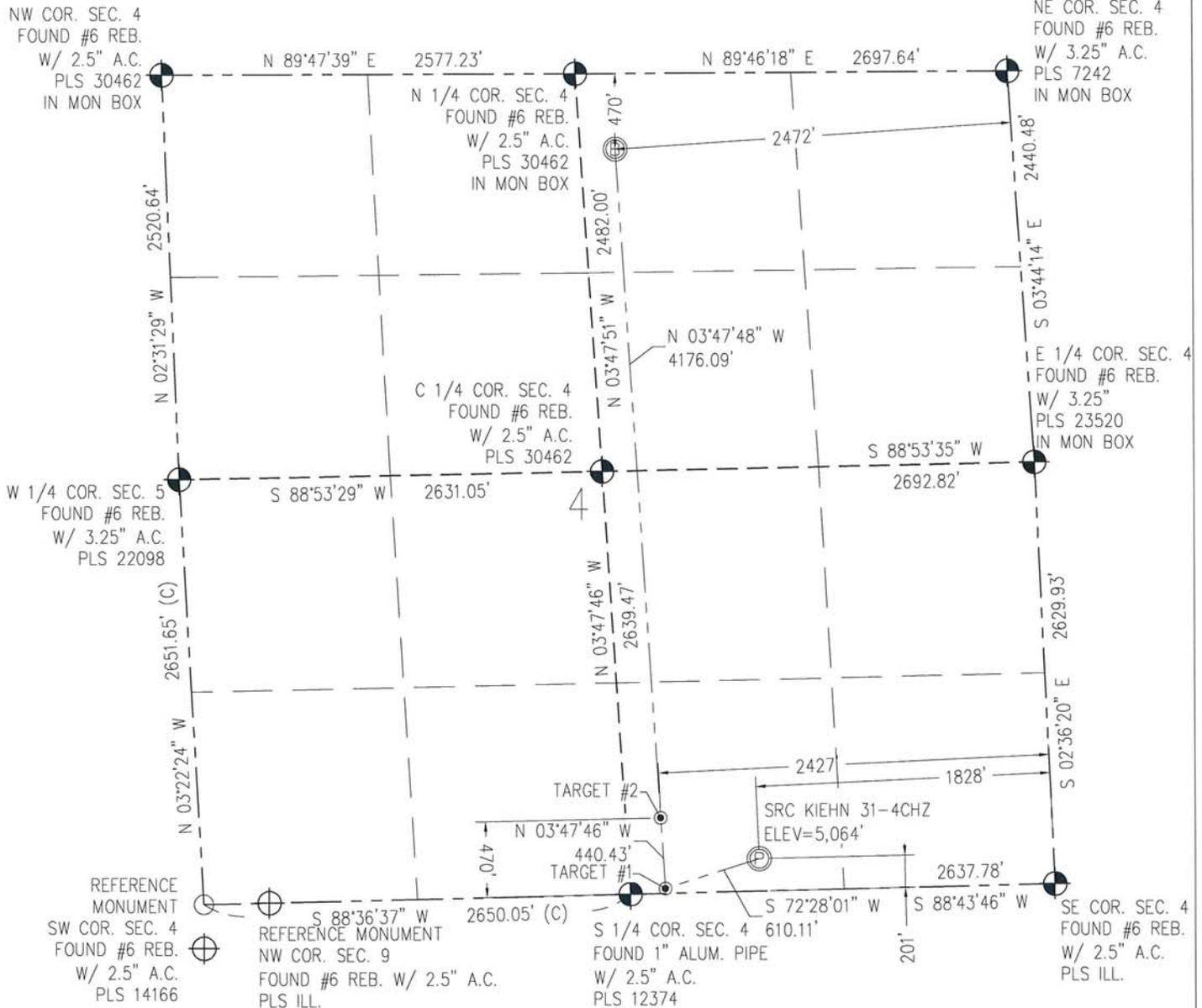
IN ACCORDANCE WITH A REQUEST FROM CRAIG RASMUSON - SYNERGY RESOURCES, BASELINE ENGINEERING CORP. HAS DETERMINED THE LOCATION OF THE SRC KIEHN 31-4CHZ TO BE 201' FSL AND 1828' FEL, AS MEASURED AT NINETY (90) DEGREES FROM THE SECTION LINE OF SECTION 4, TOWNSHIP 4 NORTH, RANGE 68 WEST AND THE BOTTOM HOLE LOCATION TO BE 470' FNL AND 2472' FEL OF SECTION 4, TOWNSHIP 4 NORTH, RANGE 68 WEST, 6TH PRINCIPAL MERIDIAN, WELD COUNTY, COLORADO.
