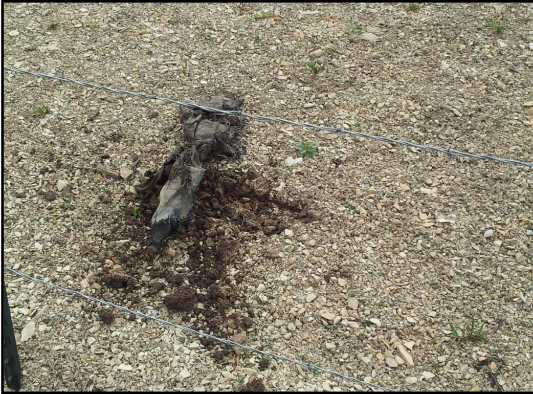
Piece of liner pulled from the ground.
